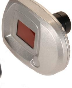
ICX404AL sensor can be set up to four seconds, however in practice I found that one second was always enough to obtain a guide star. Cross hairs can be set and a star locked into the guider, and you can even zoom in on the star to ensure you get good focus. Its auto calibration routine will be familiar to those who have previously used applications like *PHD* or *Maxim* in that it calibrates your mount's positional and set-up characteristics, and you
